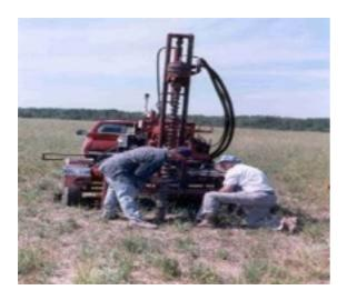
**Injection:** For soil and ground water. This is the least invasive treatment and the best method to use near buildings, especially in residential areas and places of restricted access.
